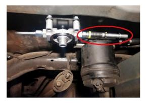
**STEP 6.** The other end of the rubber fuel hose you screwed onto the J-tube will now push and lock onto the one you just removed from the stock fuel canister. Now install and hand tighten the new filter.
