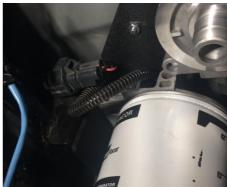
**STEP 5.** Referring to the picture below, now install the small straight tube and O-ring fitting in filter base and tighten using a 1" wrench. Once installed, spread the red locking clips on the quick disconnect right beside it and pull it straight down. This will unlock the fitting where you can now push the button on the top and pull it off the steel fuel line. Install and lock it onto the new small straight tube you just installed.
