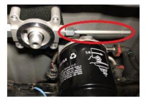
**STEP 6.** The other end of the rubber fuel hose you screwed onto the J-tube will now push and lock onto the stock one you just removed the fuel fitting from. Now install and <u>HAND</u> tighten the new filter.
