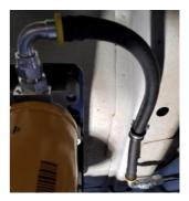
**STEP 5.** Discard the steel line you cut out and slide the nuts first and compression sleeves second onto the steel line. (NOTE: The shoulder on the compression sleeve faces the nut if it happens to fall out and you are not sure which direction it goes on the fuel line).
