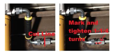
**STEP 5.** Discard the steel line you cut out. Deburr the remaining ends and slide the nuts first and compression sleeves second onto the steel line. (NOTE: *The shoulder on the compression sleeve faces the nut if it happens to fall out and you are not sure which direction it goes on the fuel line*).
