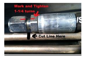
(NOTE: The shoulder, or thick end on the compression sleeve faces the nut if it happens to fall out and you are not sure which direction it goes on the fuel line).
